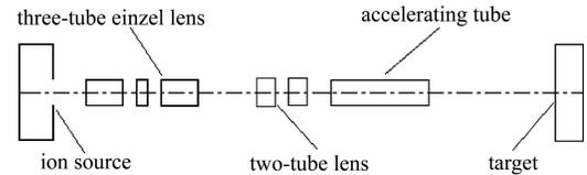
Fig. 2. Beam transport line.
