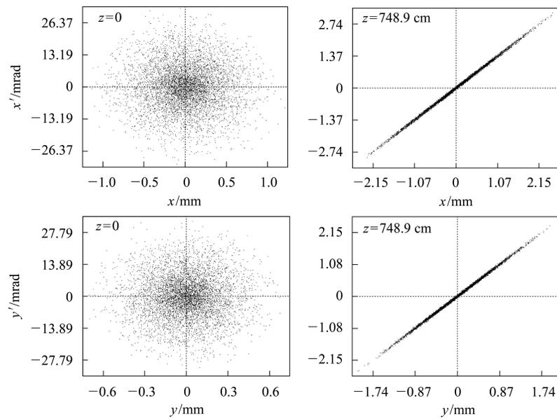
Fig. 4. Particle distribution at horizontal (upper) and vertical (lower) projection in the phase space  $I = 2$  mA.
