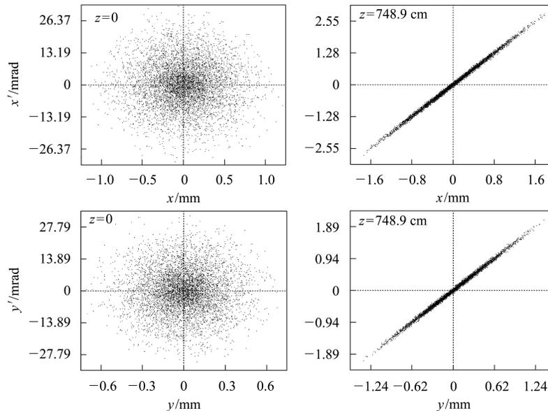
Fig. 3. Particle distribution at horizontal (upper) and vertical (lower) projection in phase space  $I=0$ .
