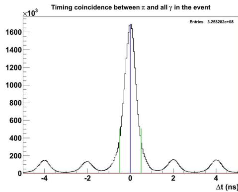
Fig. 3. Timing coincidence,  $\Delta t$ , at the event vertex between all associated photons and the pion. For each event, the photon with the lowest  $\Delta t$  is chosen, then a cut is applied at  $\pm 0.5$  ns, as shown, to remove contamination from neighbouring beam bunches.
