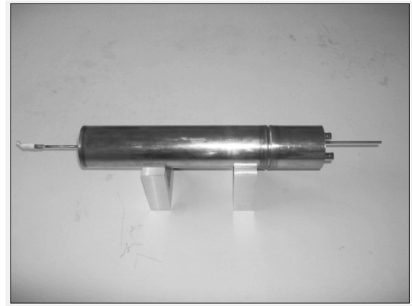
Fig. 2. The prototype ionization chamber.
