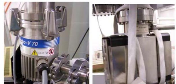
Fig. 8. The vacuum system: (left) turbo molecular pumps of 70 L/s; (right) ion pumps of 150 L/s.
