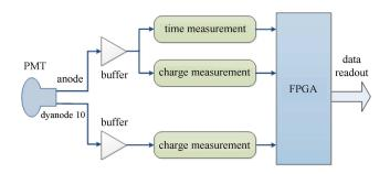
Fig. 4. Readout of the PMT signal.
