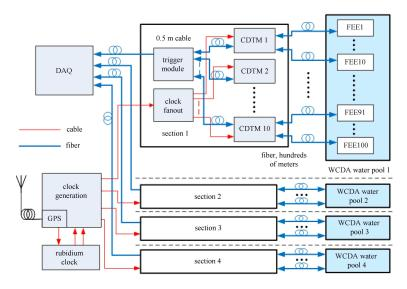
Fig. 3. Architecture of the WCDA readout electronics.
