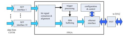
Fig. 9. Block diagram of the LHAASO trigger module.
