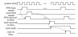
Fig. 7. Timing sequence for a global reset.
