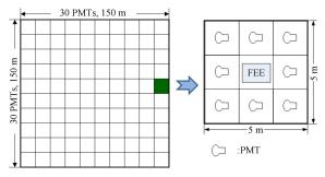
Fig. 2. Structure of one WCDA pond in LHAASO.
