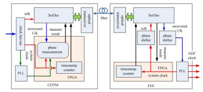
Fig. 6. Block diagram of the clock distribution and delay compensation method.
