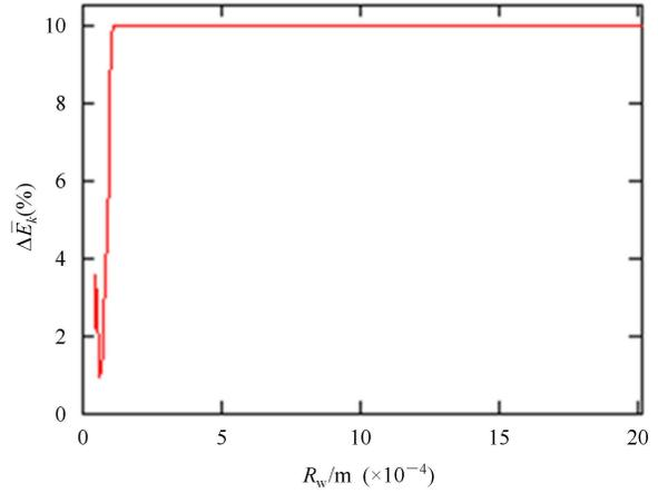
Fig. 3. (color online) Relative change in the kinetic energy of the macro-bunch versus the radius of the waveguide.
