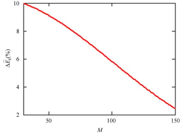
Fig. 6. (color online) Macro-bunch kinetic energy increase versus the number of micro-bunches.
