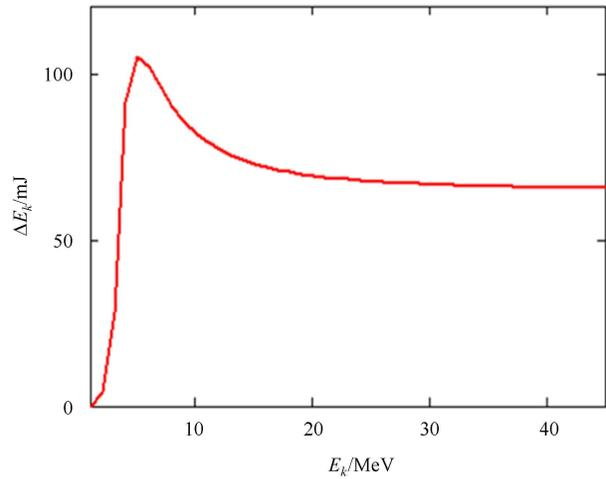
Fig. 4. (color online) Macro-bunch kinetic energy increase versus the average kinetic energy of the electrons.
