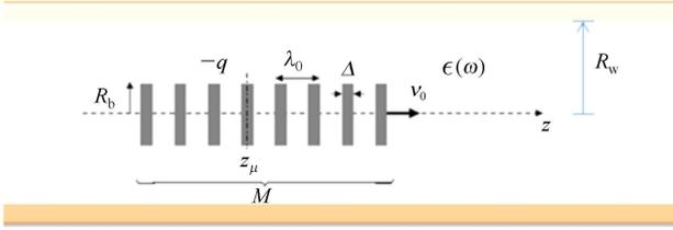
Fig. 1. (color online) Schematic of beam-active medium interaction in a waveguide.
