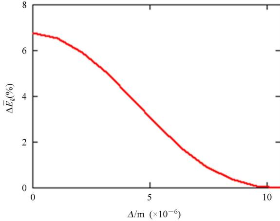
Fig. 5. (color online) Macro-bunch kinetic energy increase versus the length of the micro-bunch.
