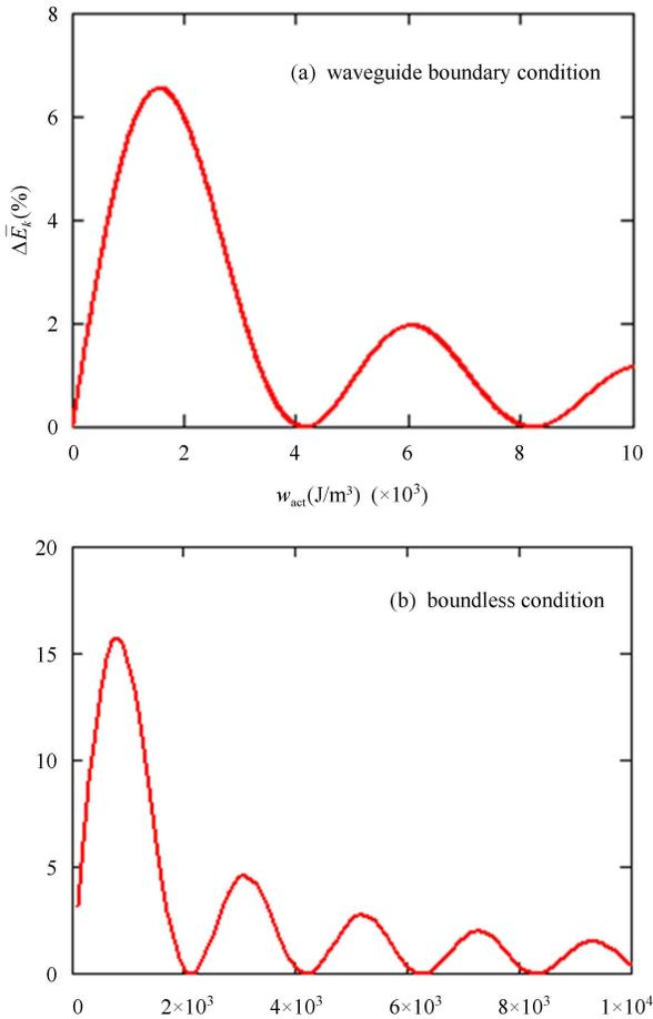
Fig. 2. (color online) Relative change in the kinetic energy of the macro-bunch versus the energy density stored in the excited CO<sub>2</sub> gas mixture.
