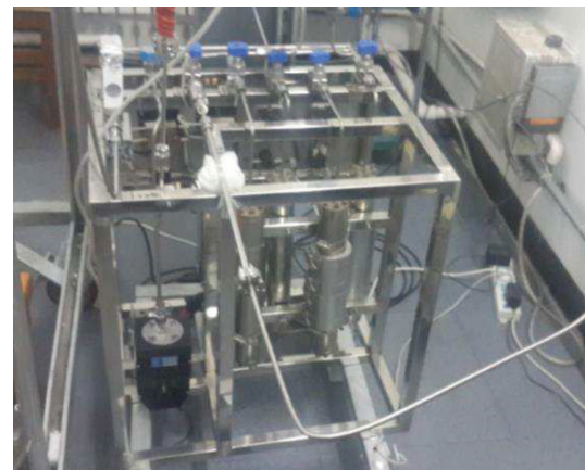
Fig. 3. Purification system, developed by Beijing Beiyang United Gas Co., Ltd, designed for reducing nitrogen, oxygen, and water impurities to lower than 0.1 ppm levels.
