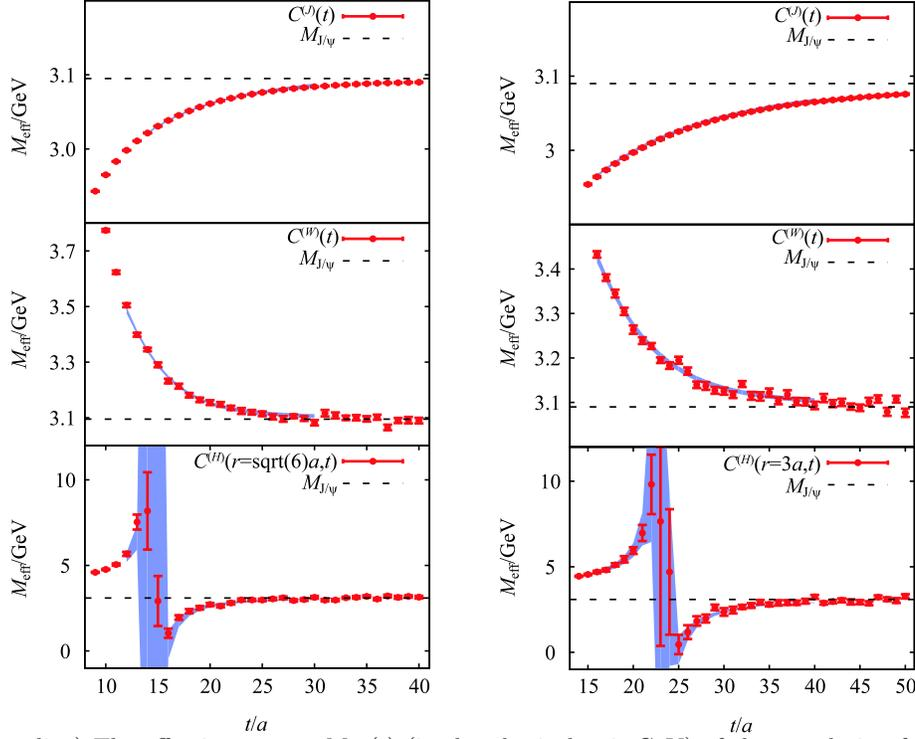
Fig. 4. (color online) The effective masses  $M_{\text{eff}}(t)$  (in the physical unit GeV) of the correlation functions  $C^{(X)}(t)$  with X standing for J, H, and W, respectively. The mass of the ground state (J/ $\psi$ ) is plotted as a horizontal line to guide the eye. We also show the effective masses (in blue bands) of the functions in Eq. (12) using the fitted parameters at  $t_{\text{min}} = 12a_t$  for  $\beta = 2.4$  and  $t_{\text{min}} = 16a_t$  for  $\beta = 2.8$ .
