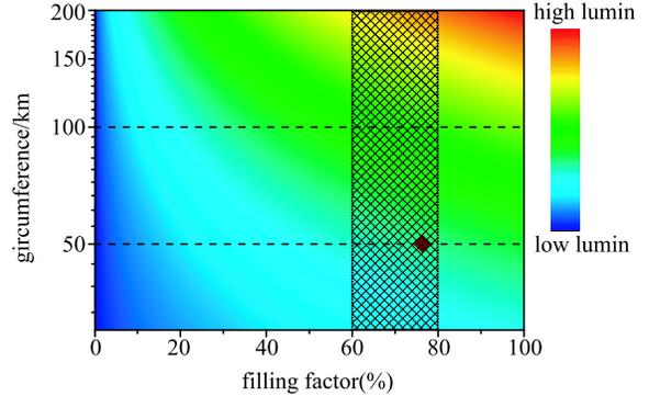
Fig. 3. The relationship of luminosity with circumference and filling factor. The shaded area shows the reasonable choice range from experience. The diamond represents the choice of 50 km CEPC design.
