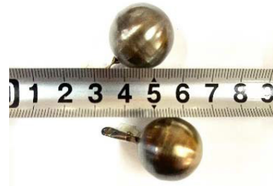
Fig. 2. (color online) Photograph of the stainless steel spherical samples used in this experiment.
