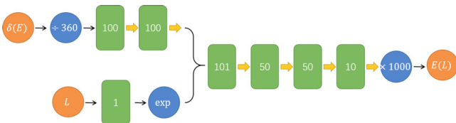
Fig. 2. (color online) The structure of our neural network. Green round rectangles with integer n represent the linear layer with size n , which consists of all the learning parameters. Orange circles denote the input and output nodes and blue circles are layers with operations marked in the middle. The yellow thick arrow marks the ‘‘SoftPlus’’ activation function and the right brace is a conjunction of the corresponding layers.
