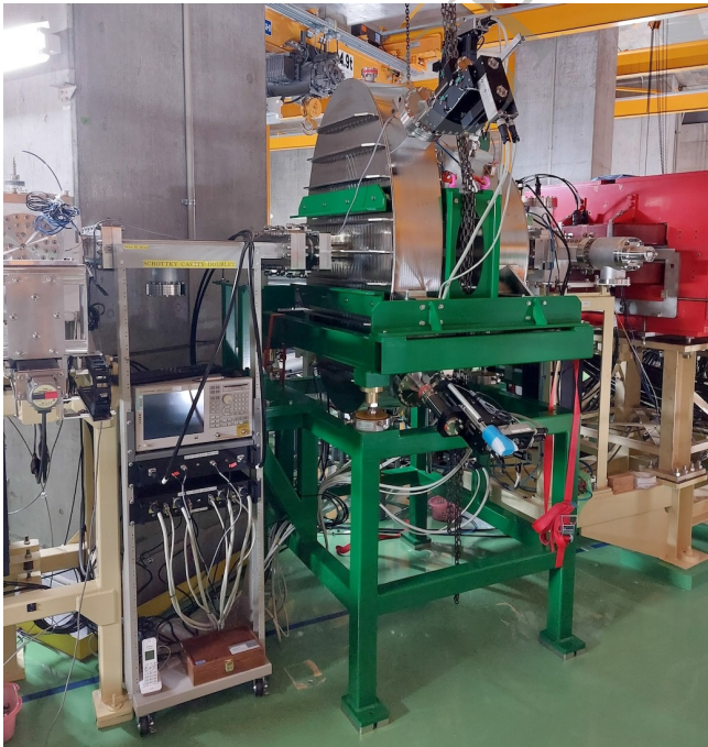
Fig. 1. (color online) A photograph of a Schottky Cavity Doublet (SCD) installed at R3 storage ring. It is shown above on top of green mechanical support (elliptical cavity left). A separate publication will be dedicated to the technical details and features of the new detector. (Photo: S. Sanjari)
