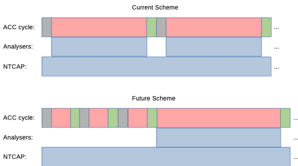
Fig. 2. (color online) Schematic of the previous timing techniques in comparison to the technique suggested by this work. Gray and green boxes show accelerator cycle start (injection) and end, red boxes show accelerator waiting time and blue boxes show recording time using the triggered spectrum analysers as well as the continuously running NTCAP.
