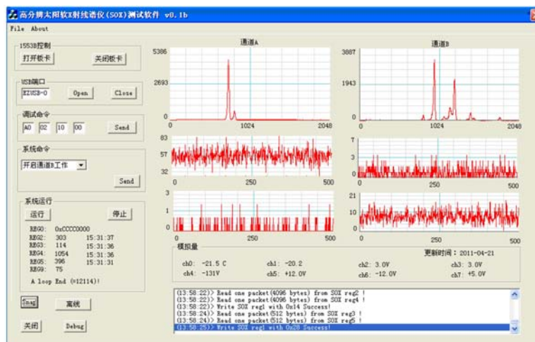
Fig. 7. The graphical user interface of the SOX ground test system.
