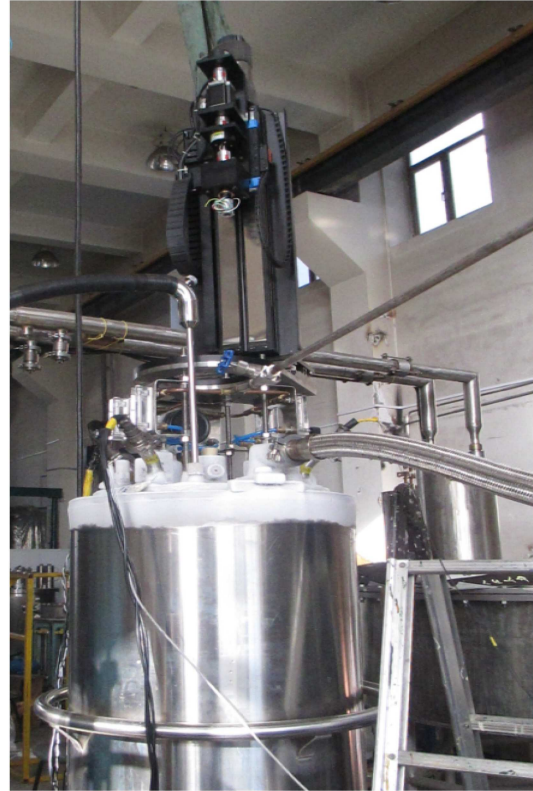
Fig. 4. Vertical test for the superconducting magnet.
